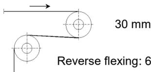
From -5°C to +8°C: add +50% on min. pulley diameter
