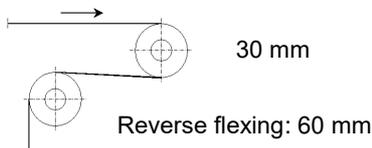
From -5°C to +8°C: add +50% on min. pulley diameter
