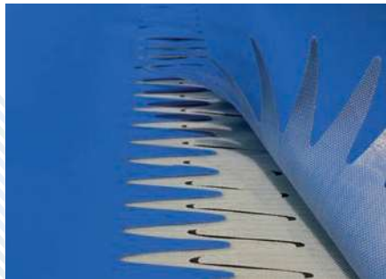
Finger overlap splicing – DS/DEC
